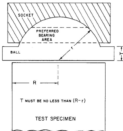
NOTE 1—Provision shall be made for holding the ball in the socket and for holding the entire unit in the testing machine.
